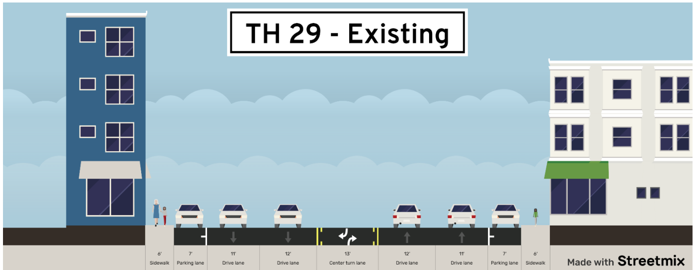
Figure 2 Existing Cross Section
